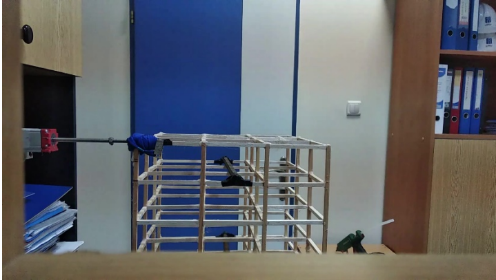
Figure 1. Displacement Meter Connection and Tracking Point
